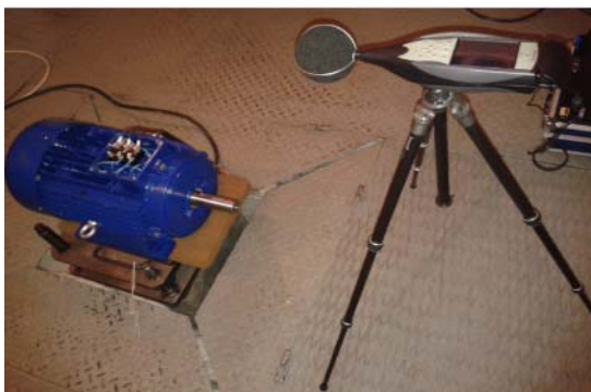
Figure 8. Experimental installation for noise level measurement by means of the Bruel&Kjaer sound-level meter.
