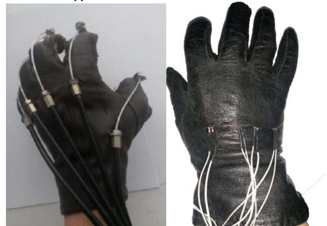
Figure 1. The exoskeleton glove with metal tendons (left) and the glove with sensors for copying the healthy hand movements (right)
