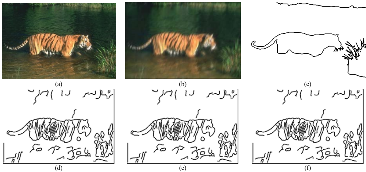
Figure 4. Selected edge detection results from Data set I using the proposed method, (a) original image, (b) blurred version of (a), (c) ground truth edges and (d-f) correspond to edge detection results produced with 3 \times 3 filter size for various \sigma values, 0.3, 0.5 and 0.7, respectively.
